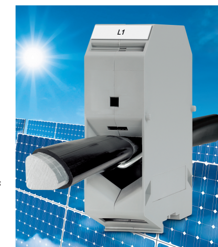
Fig. 5: Underground cables with aluminum conductors are often used to connect open land PV systems, e.g., type Navy 4 x 240 SE. This sector-shaped, single-strand aluminum conductor can be connected directly to the UKH 240 screw connection terminal block.
